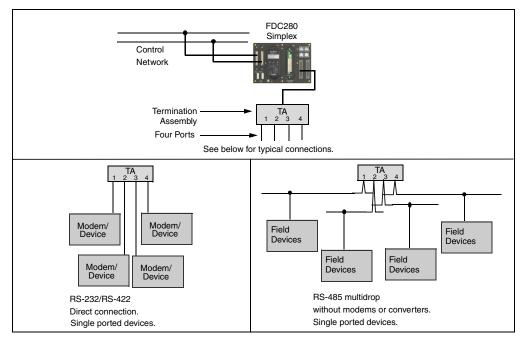
Figure 5 - FDC280 Simplex in Typical Serial Network Configurations
