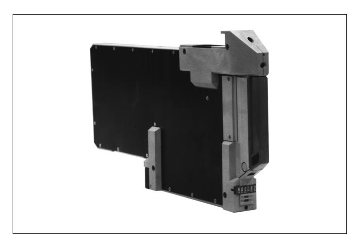
The Control Processor 30, Style B is an optionally fault-tolerant station which, together with connected Fieldbus Modules, performs regulatory, logic, timing, and sequential control. It also performs data acquisition (via the Fieldbus Modules), alarm detection and notification, and may optionally serve as an interface for one or more Panel Display Stations.
