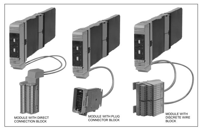
The 120 V ac Input Interface Module (an expandable main module) and its counterpart 120 V ac Expansion Input Interface Module individually function as a 16-channel 120 V ac monitor. Each module performs the signal conversion required to interface these digital (i.e., on/off state) electrical input signals from the field sensors to the redundant Fieldbus. The expandable main module independently connects to the Fieldbus and is capable of supporting a single expansion module.
