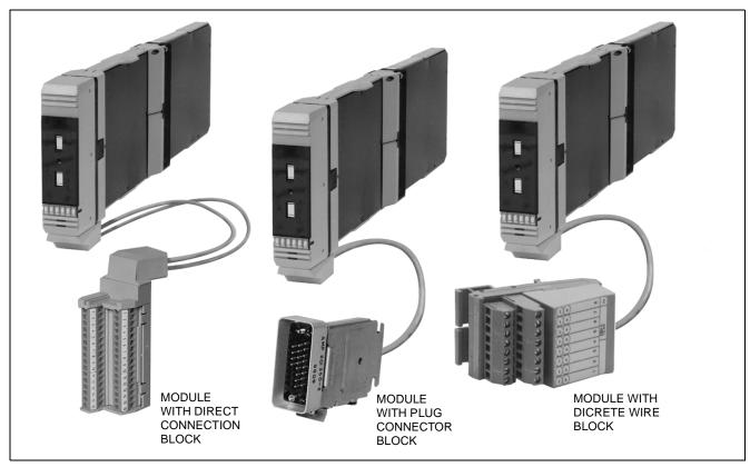
The Intelligent Transmitter Interface contains eight individual channels, each providing isolated power and communication capabilities to an Intelligent Transmitter over a single pair of wires. The module provides bi-directional digital communications between the Intelligent Transmitter and the system redundant Fieldbus.
