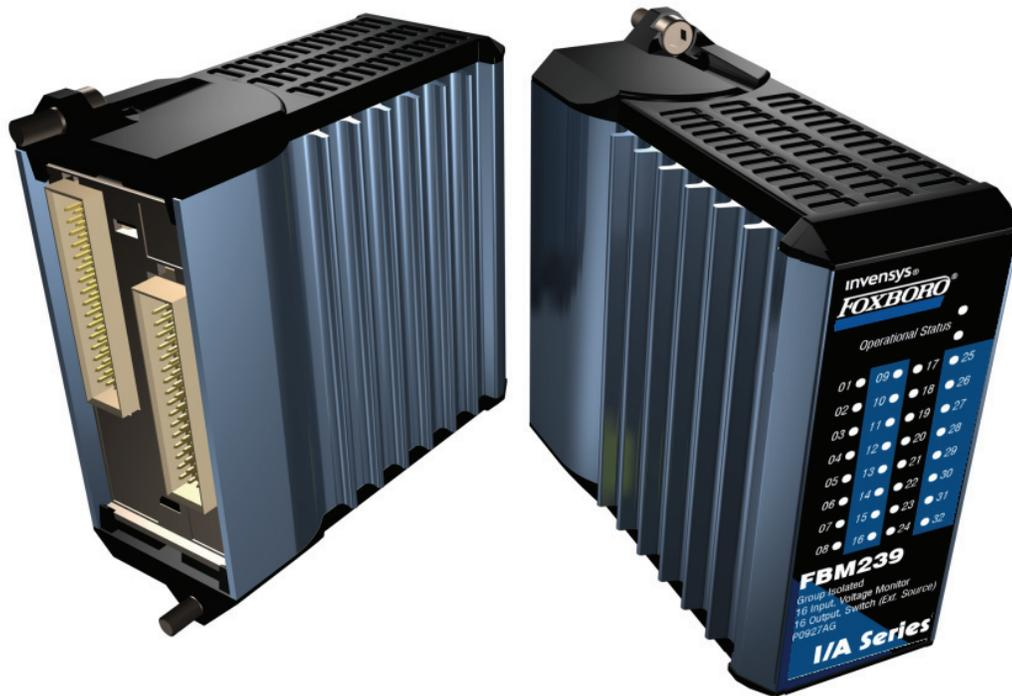
*The FBM239 Discrete 16DI/16DO Interface Module provides sixteen voltage monitor digital inputs with sixteen digital output (external sourcing) channels.*
