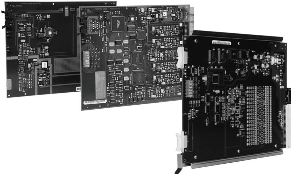
I/A Series® distributed control system (DCS) Fieldbus Modules allow migration from Honeywell TDC 2000 and TDC 3000 process I/O components to an I/A Series process control system.
