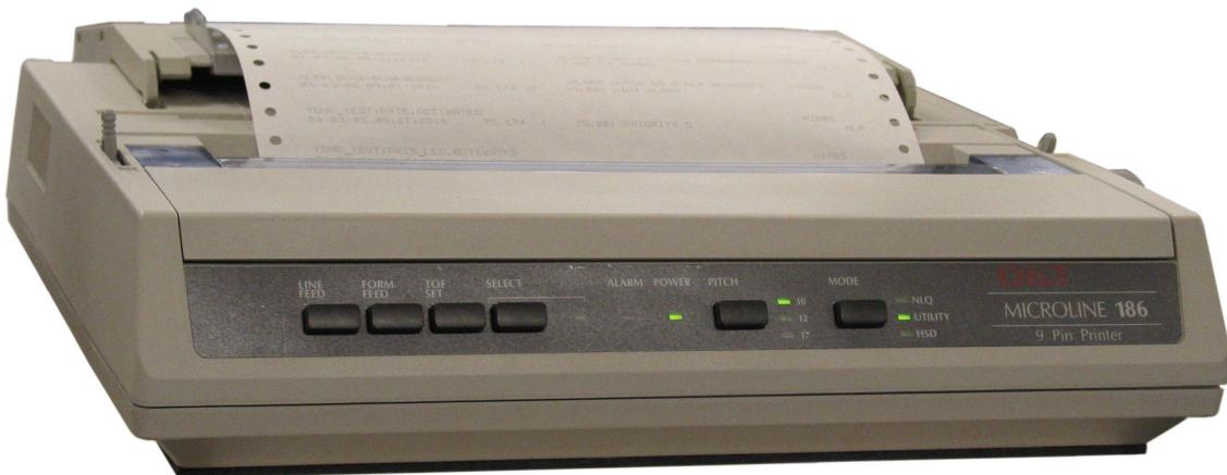
The Dot-Matrix Printer 80 is an 80 column printer for use in black/white text and graphics applications. It may be used as a log printer and may be desk- or table-mounted.
