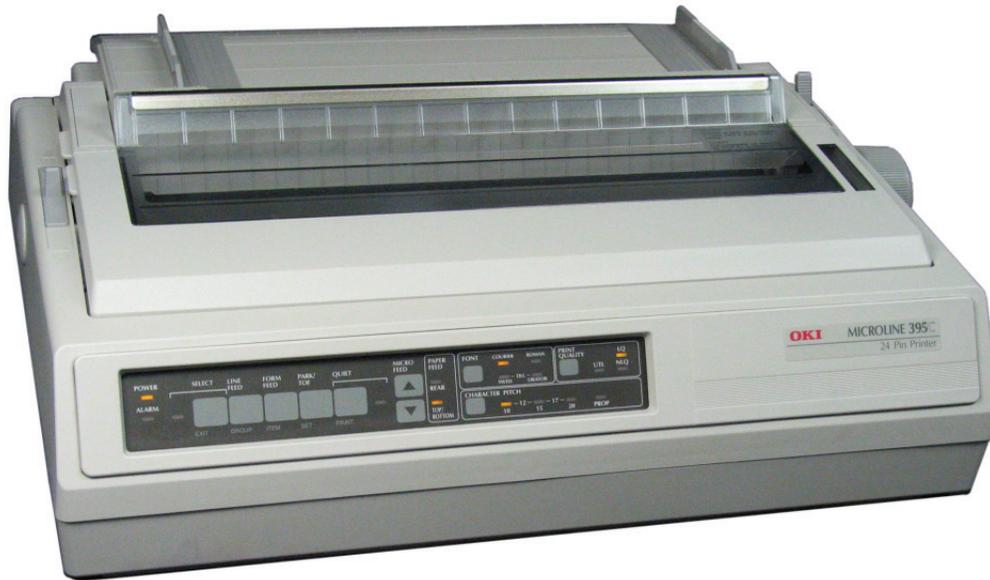
*The 132-column color dot-matrix printer can be used as an I/A Series® system log or alarm printer.*
