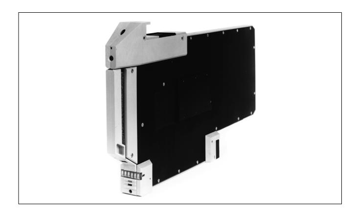
The Workstation Processor 30, together with its connected peripheral devices, provides a link between the user and all system functions. It receives graphic and textual information from application processors and other system stations and generates video signals to display the information on a video monitor.
