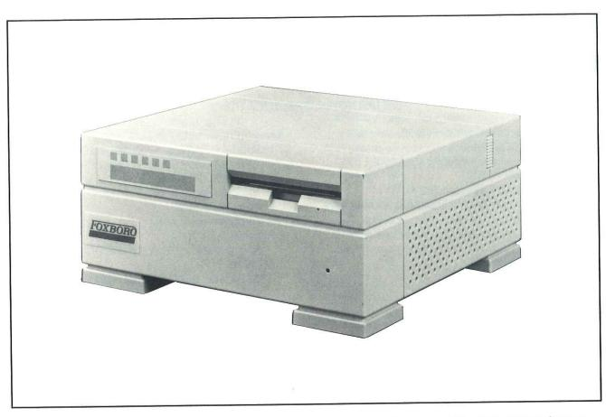
The Workstation Processor 51, together with its connected peripheral devices, provides a link between the user and all system functions. It receives graphic and textual information from application processors and other system stations and generates video signals to display the information on a video monitor.
