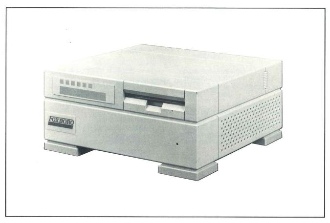
The Application Workstation 51 Processor performs application functions and workstation functions in an Application Workstation 51 subsystem. Application functions performed include:
