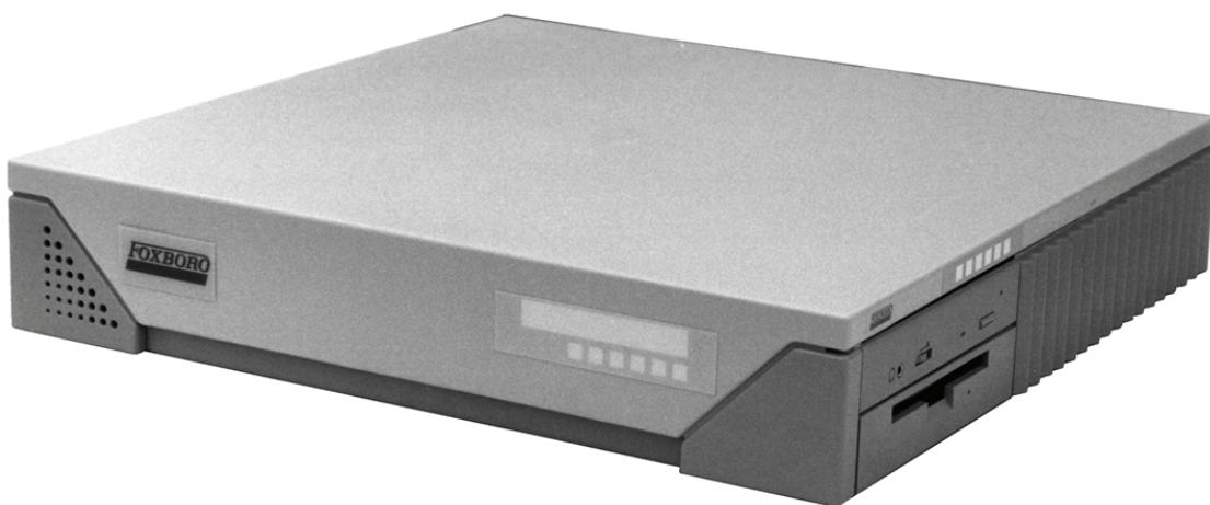
The Application Workstation 51 (AW51) Style C Processor in conjunction with its peripherals performs both application functions and workstation functions. The AW51 Style C Processor provides a higher performance level than the AW51 Style B Processor as well as boot hosting and System Monitor support for up to 64 I/A Series stations.
