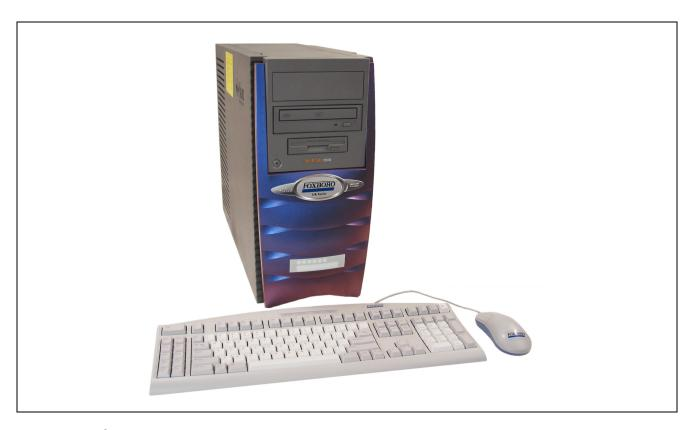
The I/A Series<sup>®</sup> Model P80 workstation is based on an UltraSPARC<sup>®</sup> III processor with a Solaris<sup>®</sup> 8 operating system. The UNIX<sup>®</sup> based Model P80 workstation in conjunction with I/A Series model-coded station software licenses and peripherals performs both application functions and workstation functions.
