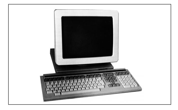
The VT100 Compatible Terminal is a software programming tool for providing high-quality alphanumeric displays for readable 80 and 132 column formats. Thirty function keys control the programming function.
