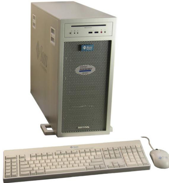
*The P82 Solaris™ Based Workstation provides a high performance, robust platform for I/A Series® application and workstation functions.*
