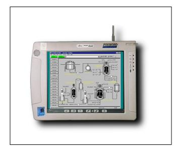
The fully integrated Mobile Workstation allows you to exchange information with your I/A Series system and/or corporate network while you are on the move throughout the plant – no strings (or wires) attached.
