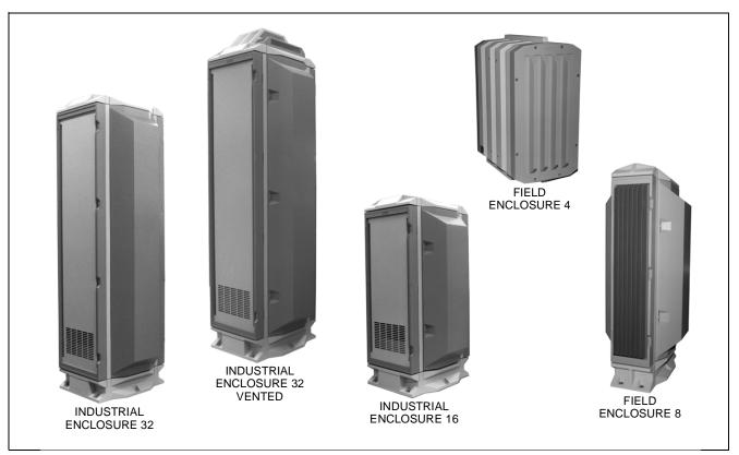
The I/A Series system structural foam enclosures extend the modular design of the system by providing a range of mounting capacities to match the application requirements. The innovative design of the packaging allows the control processor and Fieldbus Modules to be distributed closer to the process without the need for special environmentally conditioned control or equipment rooms.
