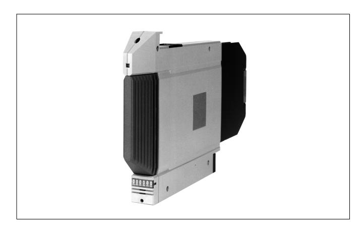
The Communications Processor 10 is a station on the I/A Series System network providing interconnection of peripherals such as a terminal I/O device, or a printer device. It has four RS-232-C compatible serial ports with asynchronous channel performance up to 9.6 kbps, or one RS-232-C compatible port with synchronous channel performance up to 64 kbps.
