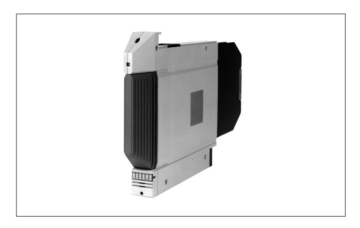
The Communications Processor 10 is packaged as a non-expandable single width X-Module which connects to the Mounting Structure Bus and accesses the Nodebus. Peripheral connections are made via cable connectors secured to the top or bottom of the mounting structure that houses the communications processor. The processor hardware architecture consists of the following:
