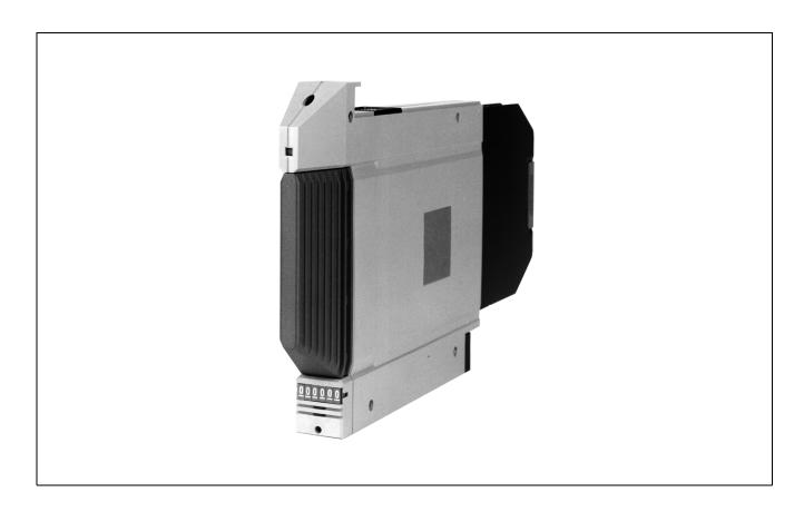
The Communications Processor 15 comprises the foundation for various intelligent device interfaces, and for computer and information network connections. It is packaged as a non-expandable single width X-Module that connects to the Mounting Structure Bus and accesses the nodebus. Peripheral connections are made via cable connectors secured to the top or bottom of the mounting structure that houses the communications processor. The processor hardware architecture consists of the following:
