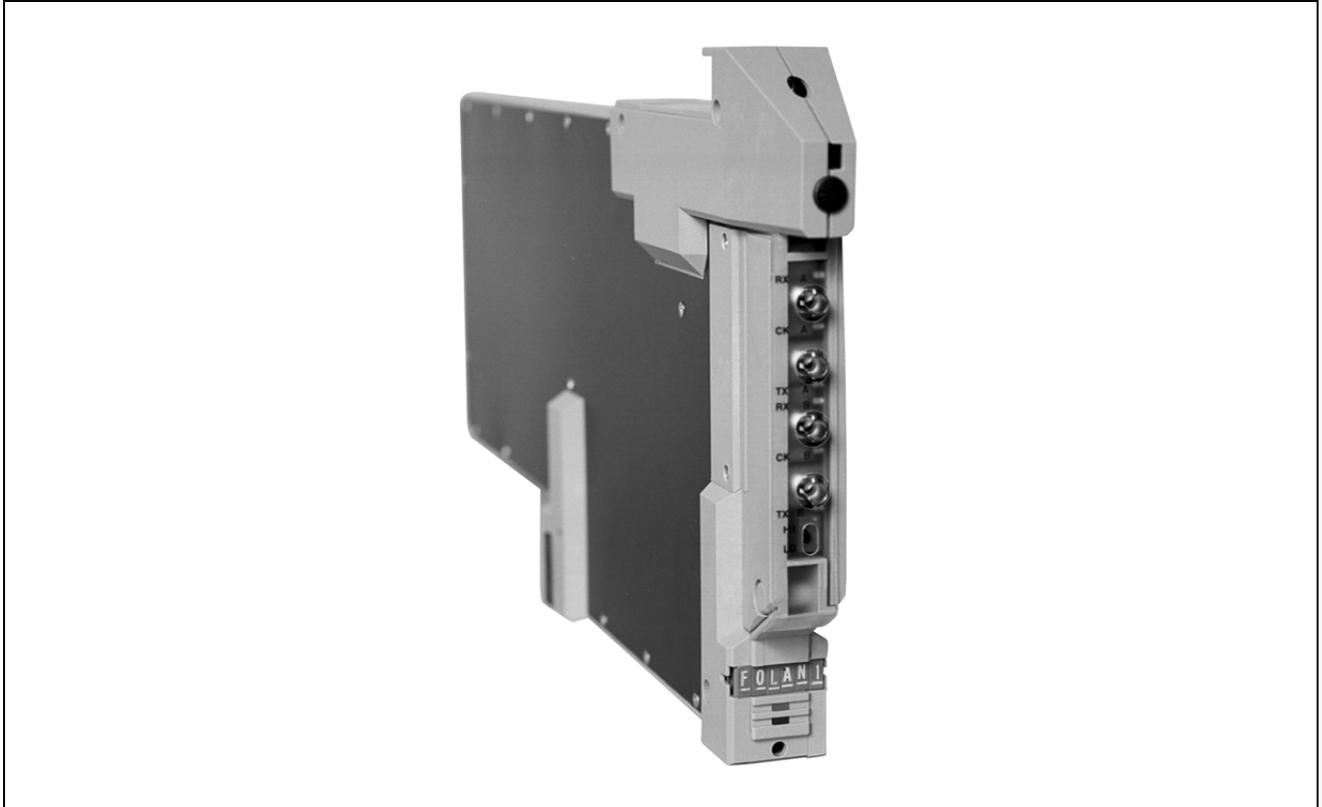
The Fiber Optic Carrierband LAN Interface module is an I/A Series Station which provides a communication interface between the Fiber Optic LAN and the I/A Series Nodebus. Packaged as a Z-module for installation in I/A Series enclosures, the Fiber Optic Carrierband LAN Interface connects to the Fiber Optic LAN cable system with two duplex fiber cables.
