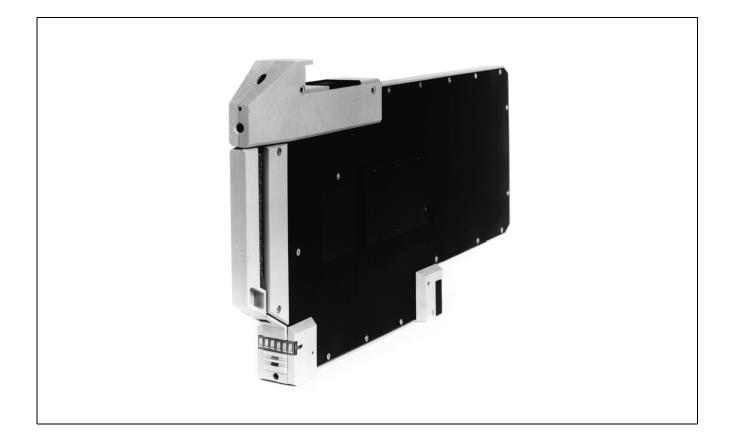
The Integrator 30 comprises the foundation for various intelligent device interfaces, and for computer and information network connections. It is packaged as a non-expandable single width Z-Module that connects to the Mounting Structure Bus and accesses the nodebus. Peripheral connections are made via cable connectors secured to the top or bottom of the mounting structure that houses the Integrator 30. The integrator hardware architecture consists of the following:
