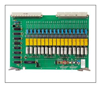
The 16 Analog Input module is a full-size electronic board in the I/A Series RTU 20 designed to read and convert 16 analog inputs from the field.
