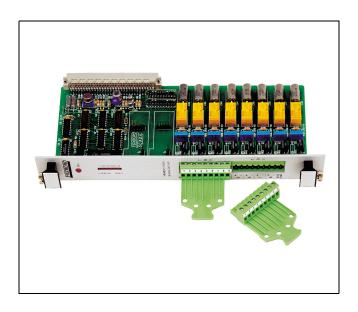
The 6 Analog Input/Reference Voltage module is a half-size electronic board in the I/A Series RTU 20 designed to read and convert 6 analog inputs from the field.
