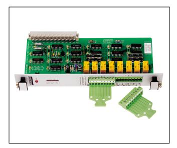
The 8 Permanent Digital Output module is a half-size electronic board in the I/A Series RTU 20 designed to drive 8 steady digital outputs through voltage-free bistable relay contacts. Field devices can be directly driven by on-board relays having gold-plated output contacts and an expected lifetime of 10<sup>7</sup> operations. Each relay provides a 1500 Vrms coil contact isolation.
