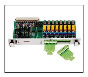
The 8 Analog Input module is a half-size electronic board in the I/A Series RTU 20 designed to read and convert 8 analog inputs from the field.
