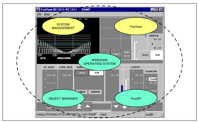
Versatile WINAPP software on a workstation for Windows provides a scalable application workstation matched to the requirements of control systems utilizing I/A Series Nodebus or Ethernet networks. The WINAPP software installs on the I/A Series Workstation Model P94 for Windows. This workstation can interface to I/A Series control stations, programmable logic controllers (PLCs) and other devices (refer to PSS 21H-4D12 B4).
