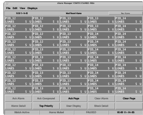
Figure 8. Example of 5-Column 10-Row Format for the Most Recent Alarms Display
