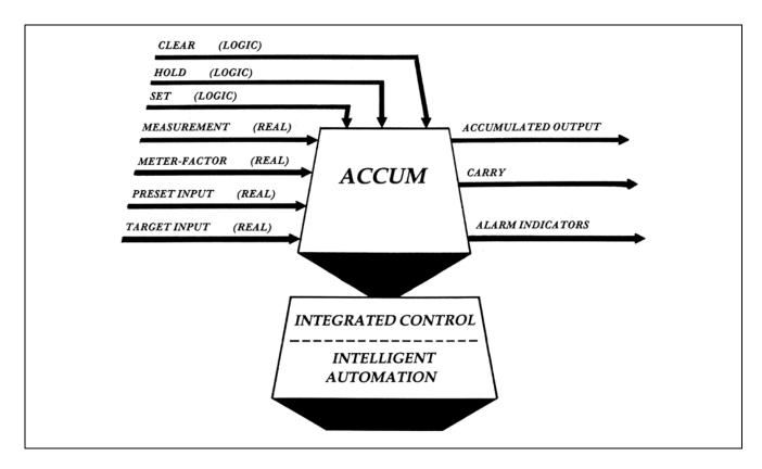
The Accumulator (ACCUM) block serves as an integrator/totalizer for monitoring flow and shutting off flow at a specified total volume, blending, etc.
