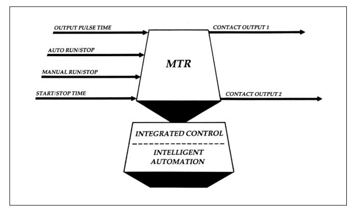
The MTR Control block provides control of 2-wire or 3-wire motor circuits. The 2-wire configuration uses a single sustained output and the 3-wire configuration uses two pulsed outputs.
