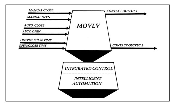
The MOVLV block provides control of a 3-wire motor operated control valve. The 3-wire configuration provides two pulsed outputs.
