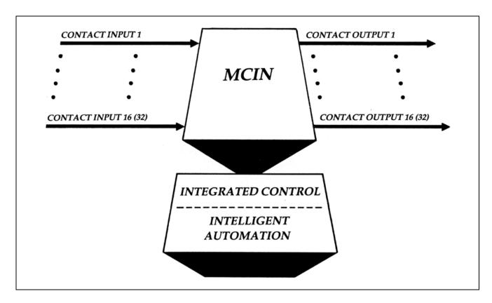
The Multiple Contact Input (MCIN) block is a multiple channel digital signal contact or logic input block for alarms and other actions on a variety of process contact or logical signal inputs.
