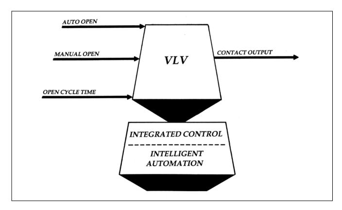
The VLV block provides open/close control of motor or air-operated valves. The block supports a 2-wire configuration using a single sustained output.
