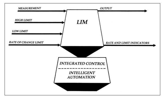
The positional/rate Limiter (LIM) block is a signal positional/rate limiter for high-low absolute and rate-of-change limiting of the measurement input.
