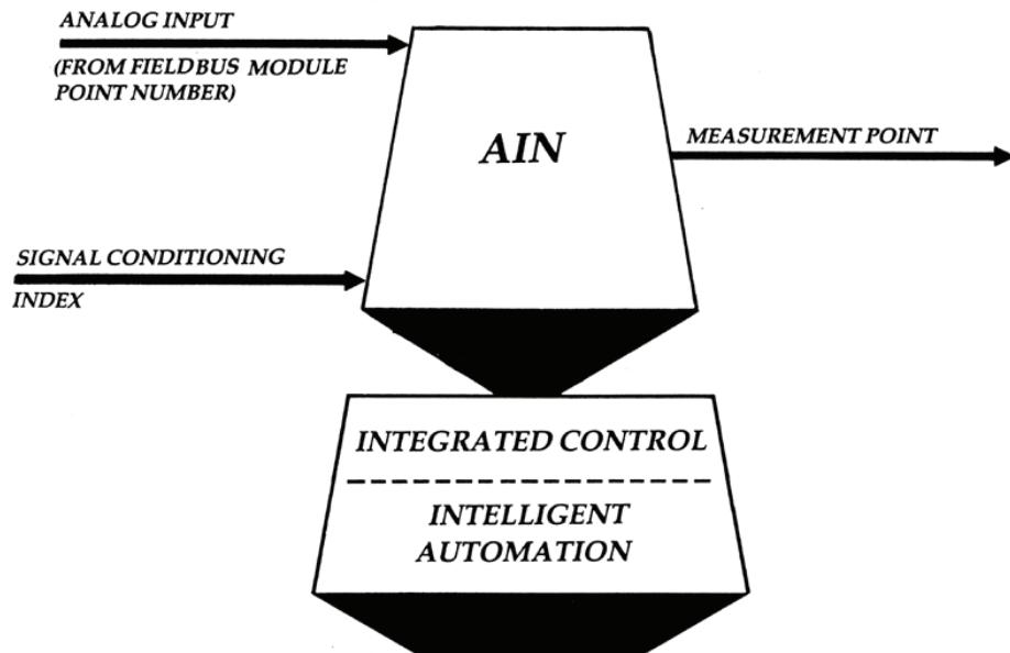
The Analog Input (AIN) block is a single channel (point) signal conditioning block for scanning, filtering and alarm implementation of a field measurement.
