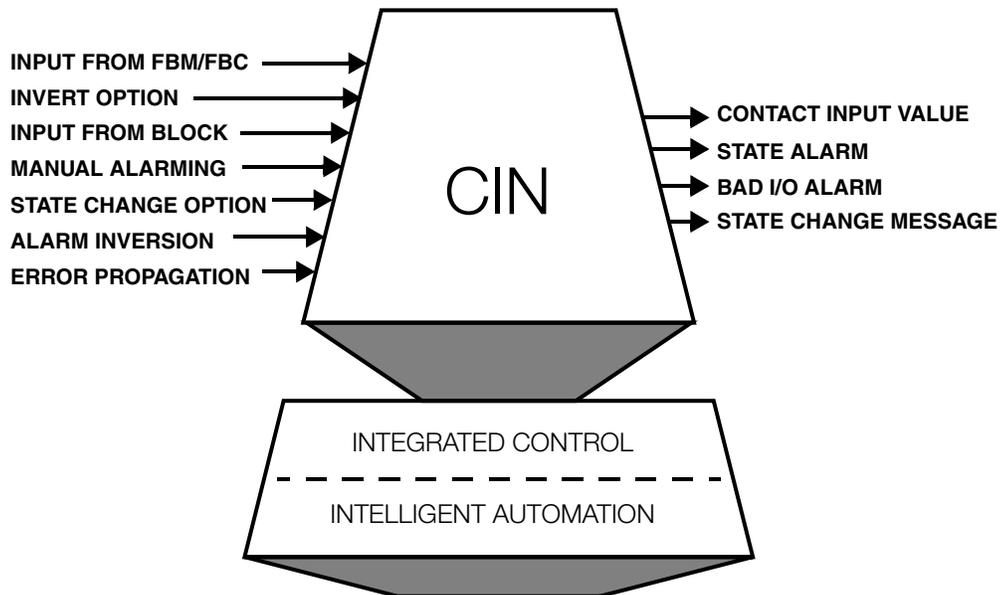
The CIN block provides input capability for a single digital input point from any Fieldbus Module or Fieldbus Card containing such points. Readback values from digital output points may also be read by the CIN block. The state of the point is made available to the control scheme as parameter Contact Input (CIN). It may represent any process contact or discrete logic input.
