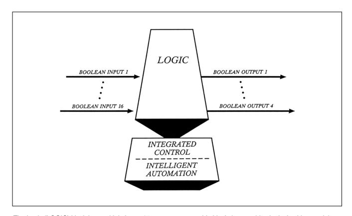
The Logic (LOGIC) block is a multiple input, 15-step, programmable block that provides logic, latching, and timer functions to augment the operation of standard blocks.
