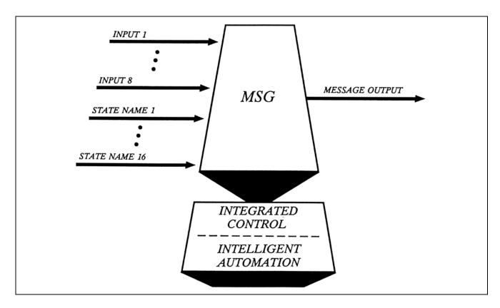
Message Generator (MSG) block generates state change messages for Intelligent Field Devices and control schemes requiring simple message generation.
