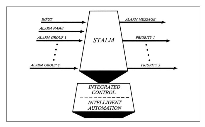
The State Alarm (STALM) block provides state alarming for event changes detected by Intelligent Field Devices and for control schemes requiring state alarming capabilities.
