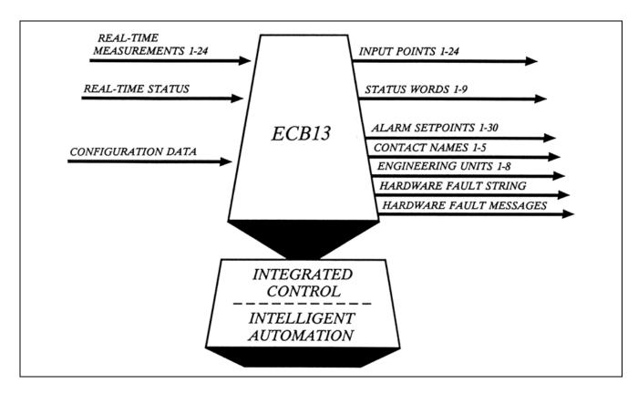
The Window Equipment Control Block (ECB) supporting the Hydrostatic Tank Gauge directly receives HTG measurement values, status conditions, and select configuration data for input to process monitoring.
