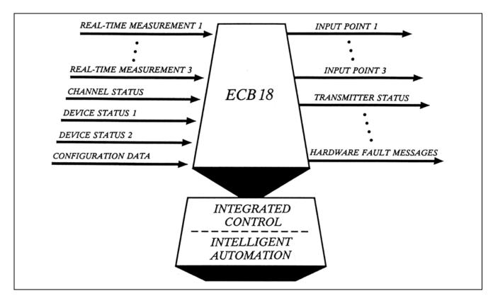
The window Equipment Control Block (ECB) supporting an Intelligent Transmitter receives measurement values and status conditions from the device for integration into the control scheme.
