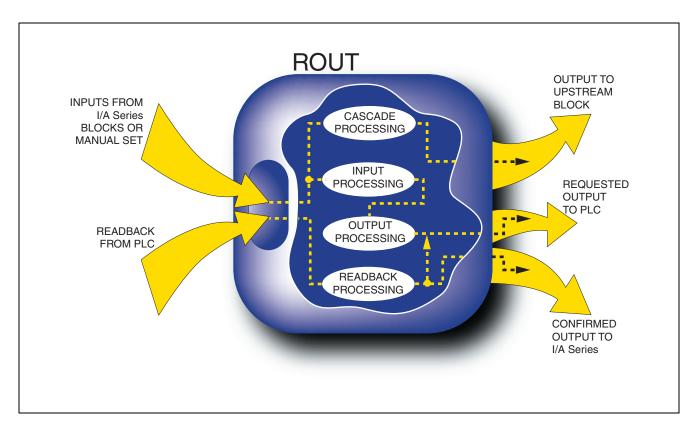
The Real Output (ROUT) block provides the control strategy with the capability to pass a single analog value to an address in an Allen-Bradley<sup>TM</sup> Programmable Logic Controller ( $PLC^{TM}$ ).
