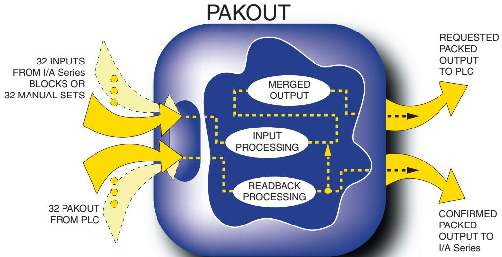
The Packed Output (PAKOUT) block provides the control strategy with the capability to pass from 1 to 32 binary values to a group of 32 contiguous addresses in an Allen-Bradley™ Programmable Logic Controller (PLC™). Each bit represents a binary value having opposing states, such as ON/OFF, or START/STOP. The data is then available for distribution to other I/A Series blocks.
