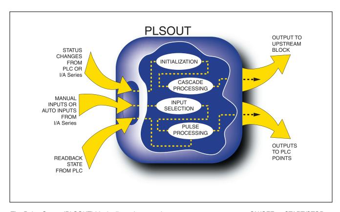
The Pulse Output (PLSOUT) block allows the control strategy or operator to output ON/OFF, or START/STOP, type commands through momentary pulsed outputs on two separate lines, one for each state, for an Allen-Bradley<sup>TM</sup> Programmable Logic Controller (PLC<sup>TM</sup>).
