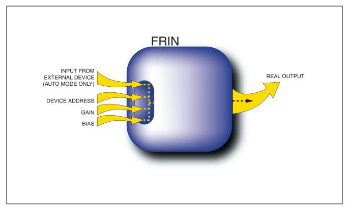
The Foreign Device Real Input (FRIN) block provides the control strategy or operator interface with a single analog value received real time from a PROFIBUS<sup>™</sup>-DP or Modbus<sup>™</sup> remote I/O device via a Micro-I/A<sup>™</sup> Station, or from a foreign device via an I/O gate. The block supports Auto/Manual control.
