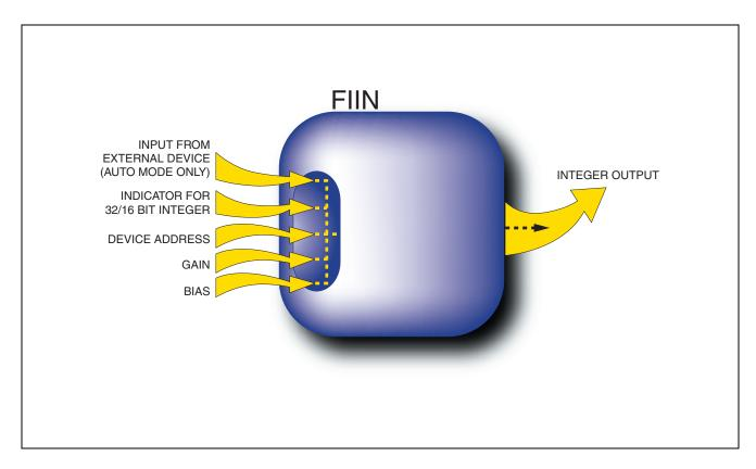
The Foreign Device Integer Input (FIIN) block provides the control strategy or operator interface with a single 16-or 32-bit integer value received real-time from a PROFIBUS™-DP or Modbus™ remote I/O device via a Micro-I/A™ Station, or from a foreign device via an I/O gate. The block supports Auto/Manual control.
