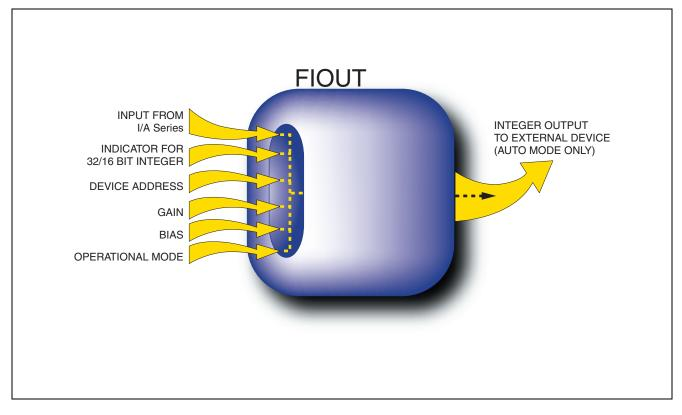
The Foreign Device Integer Output (FIOUT) block provides the control strategy with output capability for a single 16- or 32-bit integer value in real-time to a PROFIBUS<sup>™</sup>-DP or Modbus<sup>™</sup> remote I/O device via a Micro-I/A<sup>™</sup> Station, or to a foreign device via an I/O gate. The block supports Auto/Manual control.
