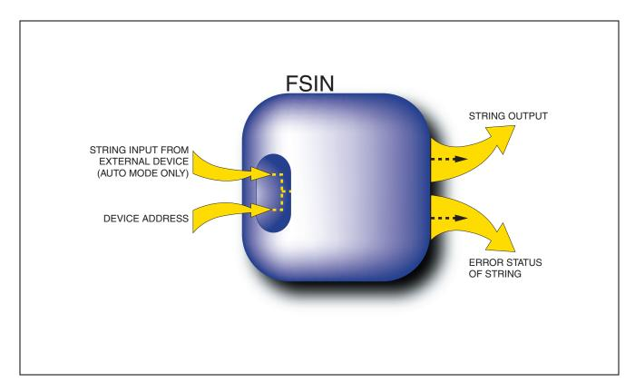
The Foreign Device String Input (FSIN) block provides the control strategy or operator interface with a single string value received real-time from a PROFIBUS™-DP or Modbus™ remote I/O device via a Micro-I/A™ Station, or from a foreign device via an I/O gate. The block supports Auto/Manual control.
