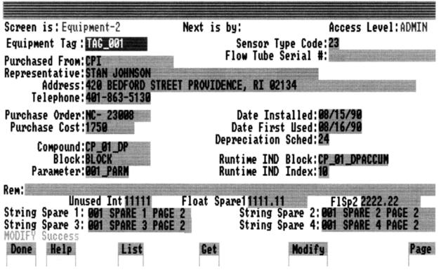
Figure 3. Equipment Information Display (Page 2) showing Intelligent Transmitter data
