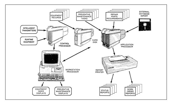
The Automation Equipment Manager is a menudriven software package which runs on I/A Series workstations and applications processors. It works in conjunction with the I/A Series Integrated Control Configurator and System Management functions to provide information needed by Maintenance Supervisors for equipment management and preventive maintenance.
