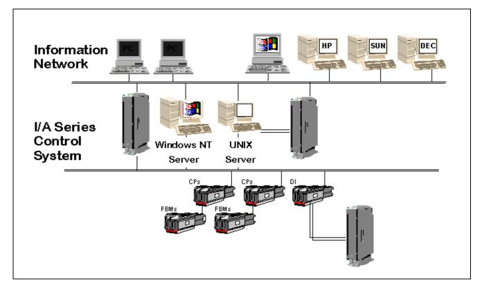
Foxboro AIM\*API and Networked AIM\*API integration software provides a consistent interface for application development and integration with the wealth of real-time and historical information supplied by I/A Series systems.
